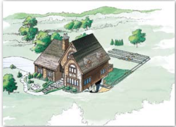
An example of a horizontal loop installation
