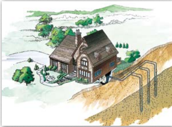
An example of a vertical loop installation
